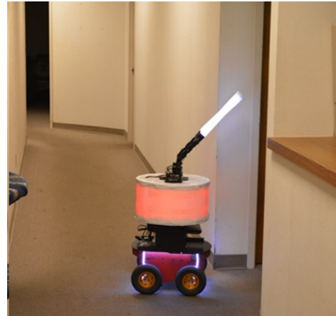
Figure 1. An emergency evacuation robot signals for the person to go to the right.
