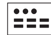
Figure 9: Class symbols can contain other symbols. This class has three field variables and six methods.
