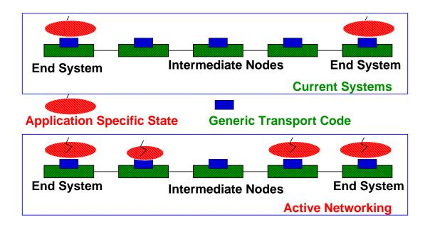
Placement and manipulation of application-specific state within the communication subnetwork.
