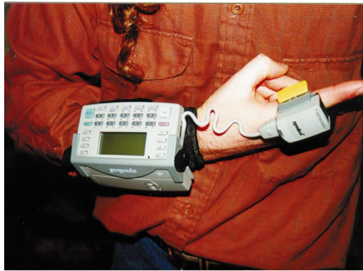
Figure 2. Symbol Technologies' wearable bar-code scanner and computer. The product is being used by United Parcel Service and has been sold to various retail chains. To date, user acceptance is high.
