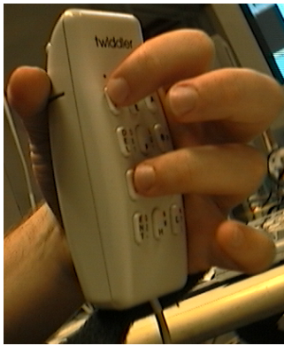
Figure 2: The Twiddler chording keyboard has three columns and four rows of buttons on the front operated by the user's four fingers. Four to six modifier keys (such as "Alt") are on the back and operated with the thumb.
