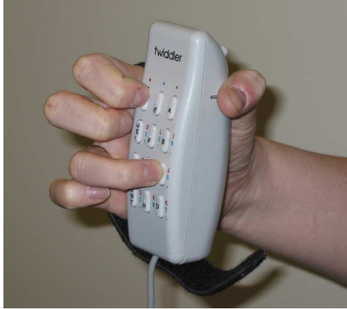
Figure 2. The Twiddler one-handed chording keyboard shown in typing position where the keypad faces away from the user.
