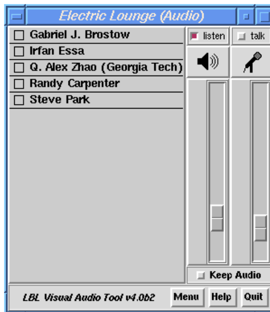
Figure 3. The audio-tool, vat. This example shows that five people are listening in the Electric Lounge. The user can mute audio from an individual participant by checking the box before the person’s name. The “listen” and “talk” check-buttons specify whether the program should play network audio and whether it should broadcast local audio signal to the network. The speaker and microphone icons indicate the devices that the program is using for audio output and audio input. The sliders adjust the volume or input gain of the audio devices.
