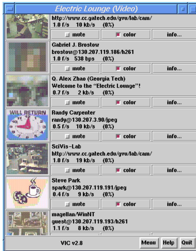
Figure 4. The original vic program. It shows the thumbnail images of all video sources as well as a few statistics associated with each video stream. Clicking a thumbnail pops up a full-size view of the video. Checking the "mute" button stops a video stream. Unchecking the "color" button lets the program to decode that particular video in grey scale.
