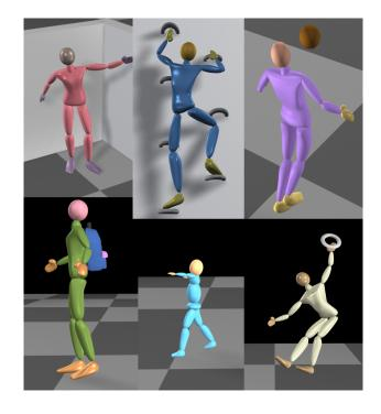
The balance controller incorporates multiple strategies for maintaining and recovering balance, including supporting the center of mass (COM), stabilizing the upper body, adjusting joint angles and velocities, taking steps and using environment features, such as walls, for support when recovering balance against large external perturbations.
