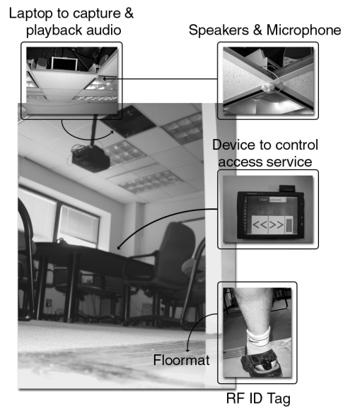
Figure 6. The conference room. Microphones and speakers are placed in the ceiling to record and playback captured audio. Floor-mats are placed at the doors to read and identify users wearing RF ID tags walking over them. Audio content is captured and tagged with the name of people present in that location for the duration of the captured audio segment.
