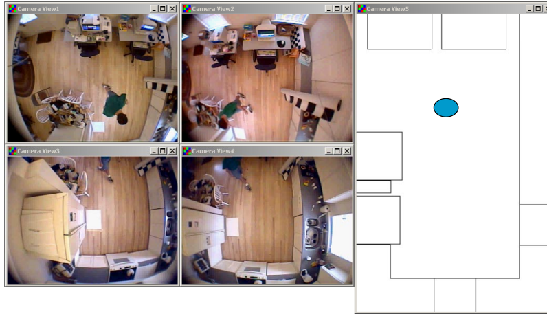
Figure 3: The visual tracking system. Four overhead cameras track moving “blobs” in the kitchen of the Aware Home. The location and orientation of these unidentified blobs is reported to the Location Service.
