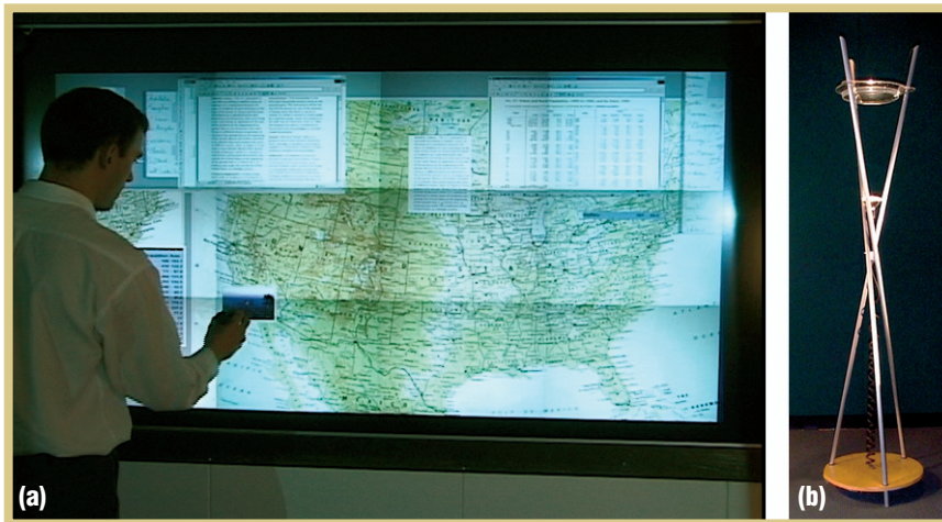
Figure 3. Form factors of ubiquitous computing. (a) The Stanford Interactive Mural—an example of a large-scale interactive display surface created by tiling multiple lower-resolution projectors. Figure courtesy of Françoise Guimbertière. (b) The Water Lamp from Hiroshi Ishii's Tangible Media Group at the MIT Media Lab—an example of an ambient display. Light shines upward through a pan of water, which is actuated by digitally controlled solenoids that can tap the water and cause ripples. External information can drive the tapping of the solenoids. Figure courtesy of Hiroshi Ishii.
