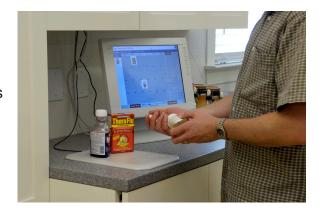
The memory mirror system uses RFID (radio frequency identification) technology. This technology is being rapidly adopted by industry as "active barcodes" for tracking inventory and tagging objects with digital information. These tags can be quite small and do not require a battery.
