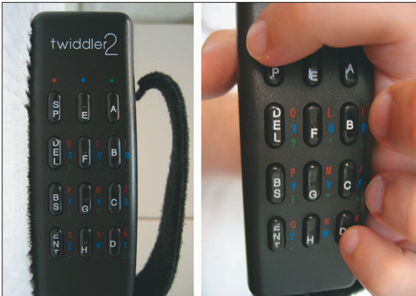
Figure 2. (a) The Twiddler one-handed chording keyboard; (b) chording the letter “k.” with the Twiddler.
