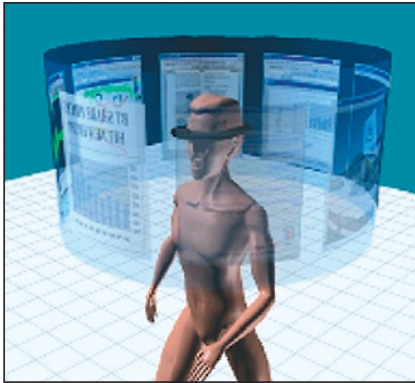
Figure 2. A head-worn display emulating a high-resolution display wrapped around the user's body. 2
