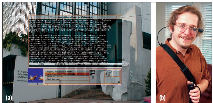
Figure 1. The MicroOptical SV-3 monocular display: (a) a simulation of the display's overlay effect; (b) the display mounted magnetically to the author's eyeglasses for quick donning and doffing.
