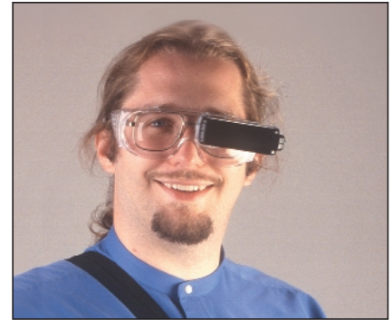
Figure 3. The Private Eye display, which is relatively large compared to today's head-worn displays.
