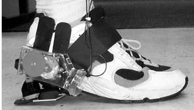
Figure 10: Rotary generator fit to a shoe for proof-of-concept studies at the MIT Media Lab.
