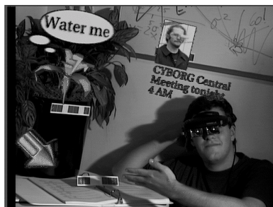
Figure 2. Multiple graphical overlays aligned through visual tag tracking. The color code of each tag provides a unique ID for the object. In addition, the vision process tracks each tag in 2.5D as the head-mounted camera moves.
