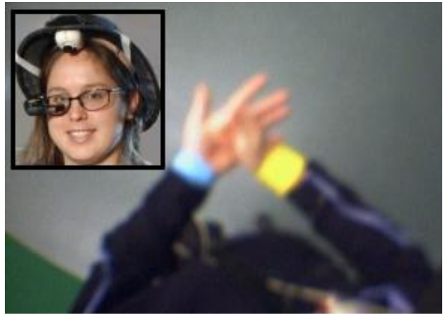
Figure 6: View from hat mounted camera with the image defocused to improve tracking. Image superimposed in the upper-left corner shows the participant wearing the hat-mounted camera along with a head-mounted display on her glasses. Note the downward-facing camera mounted beneath the brim of the hat and the head-mounted display over the left eye.
