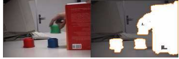
Figure 9: Experiment IV: In this frame, the book fully occludes the third peg. The system must infer the interactions that are hidden.
