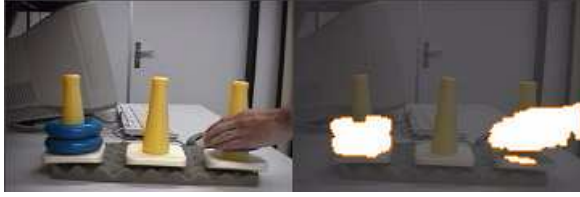
Figure 7: Experiment II: All of the discs have the same size and shape. Also, note that the dark shadow under the hand is labelled as noise
