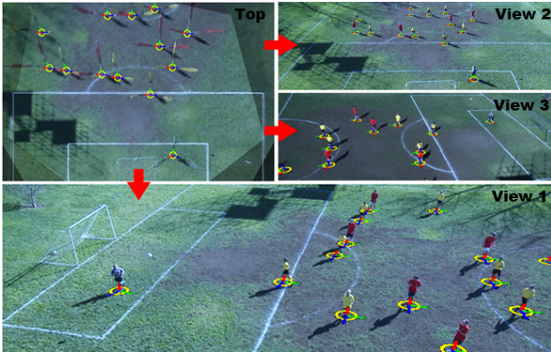
Figure 13. Evaluation of automatic player location on the ground: We back-project the position onto each view for evaluation. Each R, G and B line with yellow circle denotes the direction of the vertical vanishing points for each view (geometric constraints).
