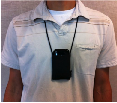
Figure 2. Our simple yet practical setup for data collection: A neck identity holder fitted with a smartphone with our custom data collection application. No specialized or expensive hardware is needed.
