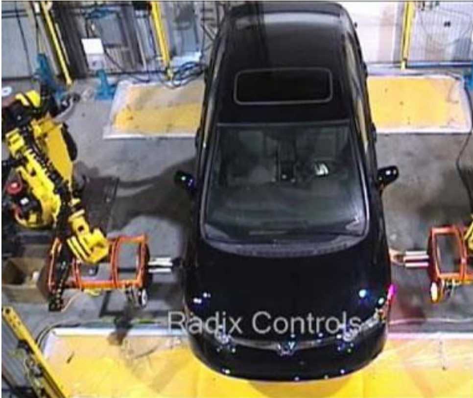
Vision-guided robots position nut runners on wheels
