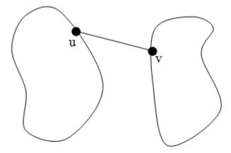
Figure 3: The lowest-cost edge happens to be between u and v. Then this edge is the lowest weight within some cut, as shown.
