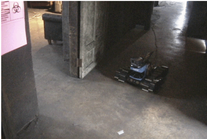
Figure 11: Urban robot following hallway inside burn building at MCPSTA, searching for biohazard indication.
