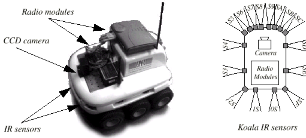
Figure 47: Koala robot used for teleoperation with haptic interface.
