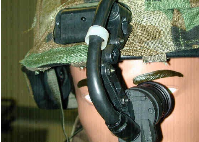
Figure 38: Early Land Warrior helmet mounted display that clearly exhibits some of the features to be avoided.
