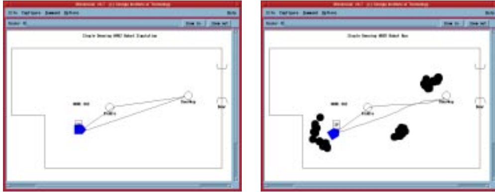
Figure 2: Left: Simulated Run on Denning Robot. Right: The same code executed on actual Denning Robot
