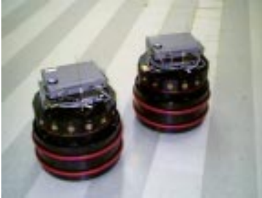
Fig. 8. Shannon and Sally, the two Nomad 150 robots used in formation experiments.
