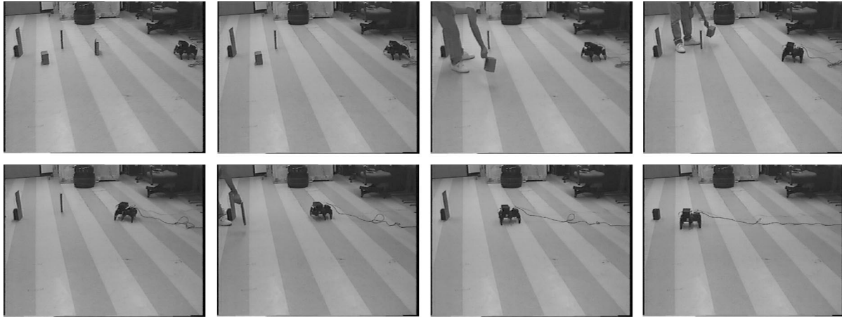
Fig. 17. This sequence of pictures depicts Miguel's reactions to many different stimuli, including when they are all simultaneously visible. The sequence proceeds from left to right. At first, all the stimuli are visible, and Miguel remains motionless because of the presence of the predator. Once the predator is removed, Miguel is moving towards the prey, both when it is stationary, and when it is moving. The prey is then removed, and Miguel tracks the mate. After the mate is removed, Miguel is moving towards a hiding-place. And, in the last picture, Miguel is just moving-forward since all stimuli have been removed from the view.
