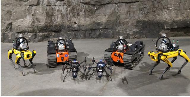
Fig. 7: The heterogeneous multi-robot team of Team CSIRO Data61 for the DARPA Subterranean Challenge Final Event: two BIA5 OzBot ATRs (tracked robots), two Boston Dynamics Spots (legged robots) and two Emesent Hovermap drones.
