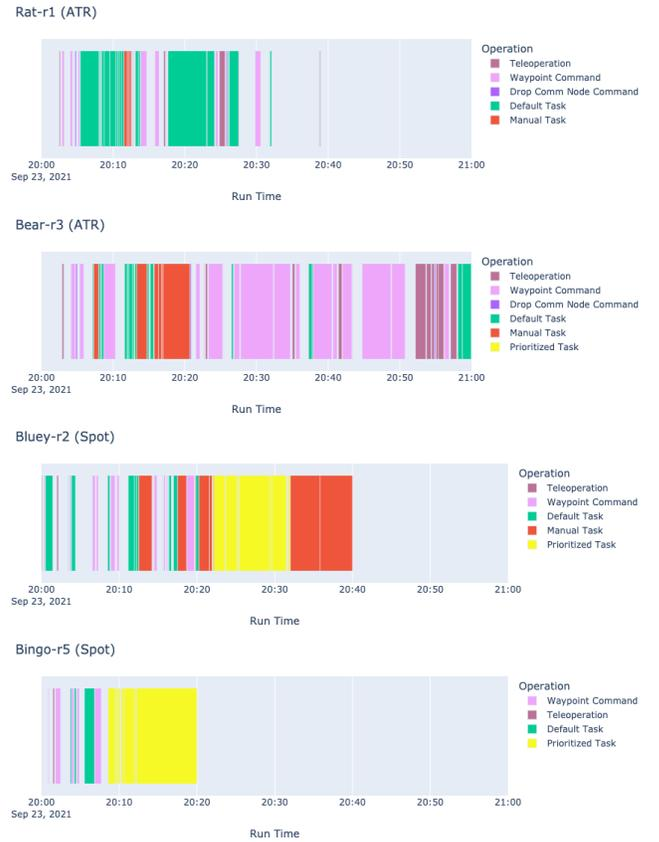
Fig. 8: The activities of each ground robot during the final run. Prioritized tasks were the tasks modified by prioritization regions; manual tasks were the tasks manually assigned to the robot by the operator, default tasks were the tasks with unchanged priorities. Note that Rat failed to operate after 40 minutes and Bingo failed to operate after 20 minutes due to inability to recover from falls.
